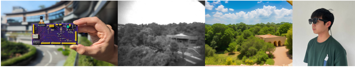
Figure 1: PixelGen argues for decoupling the camera from the mixed-reality headset. The PixelGen system captures a representation of the environment using low-resolution sensors, a monochrome image sensor and environmental sensors. The captured sensor information is then processed through a transformer-based language and image model for generating realistic representations of the environment for visualization on a mixed-reality headset.
